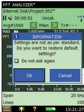
From the pop-up window for the measurement setup check (see Fig.7.3) you can set the parameters relevant for Tone Assessment to a 'default' setup that complies with the selected **Tone Standard**. To reset all relevant parameters to the preset defaults described in Table 7.1, tap on the **OK** button. To measure with the manual setup, tap on the **Cancel** button.
