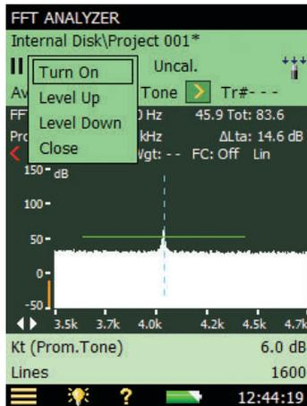
When tone generation is on the display shows the **Speaker On**
