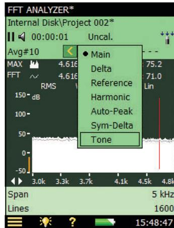
The results from the tone assessment calculation can only be displayed on the analyzer's display when the Tone Cursor is selected, see Fig. 7.5. After finishing the tone assessment calculation, the tone cursor jumps to the most prominent tone. If no tones are detected in the analysed FFT spectrum, a pop-up message will inform you that no tones have been found.
