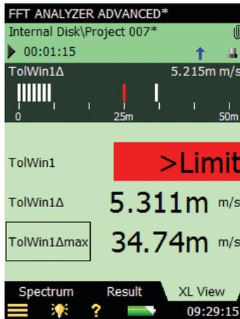
The Delta Sum parameters can be selected for display in the bar graph (tap on the parameter in first line within the bar graph). The upper limit is indicated (red line) on the bar graph together with the Max Delta Sum (a single white line). The Delta Sum parameter is displayed with the same units as the FFT spectrum.
