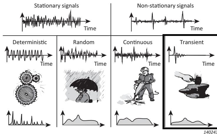
A transient signal is a signal which only exists for a short period of time. Examples of transient signals are impacts caused at industrial sites, combustion in a reciprocating machine, or the opening or closing of a valve. A transient signal produces continuous spectra.
