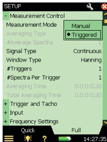
61) Set **Measurement Control** > **Signal Type** to *Transient*.
