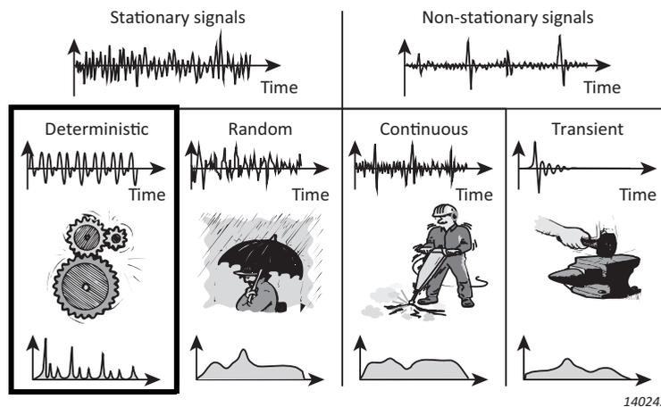
Deterministic signals are made up entirely of sinusoidal components at discrete frequencies. When the spectral lines show a harmonic relationship, the signal is described as being periodic. Examples of a periodic signals are vibration from a rotating shaft, the sound/vibration from meshing gearwheels, or more theoretically a square wave.
