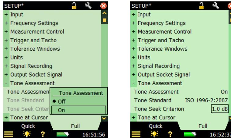
Select the **Tone Standard** as required. The **Tone Seek Criterion** is set to 1 dB by default. Increasing the criterion will make the tone seek algorithm less sensitive when searching the FFT spectrum for tone candidates. Increasing the **Tone Seek Criterion** may be relevant for analysing irregular spectra (mainly spectra with short averaging times). The **Tone Seek Criterion** can be varied between 0.5 and 4 dB.
