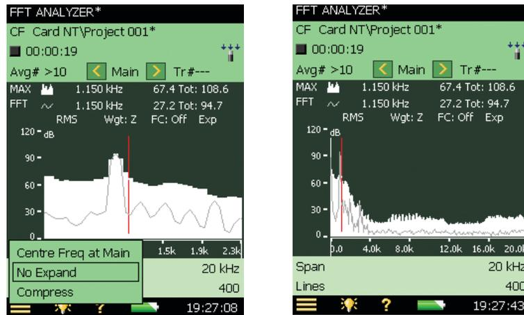
The frequency axis now displays the full frequency range (0 Hz to 20 kHz) and the spectrum is now at the default resolution again.
