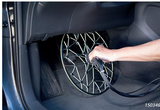
NOTE: When using the hand-held array without the reflective plate (as for acoustic holography measurements) noise will reflect off of the tablet. Remove the tablet from the holder to prevent the detection of such sounds.
