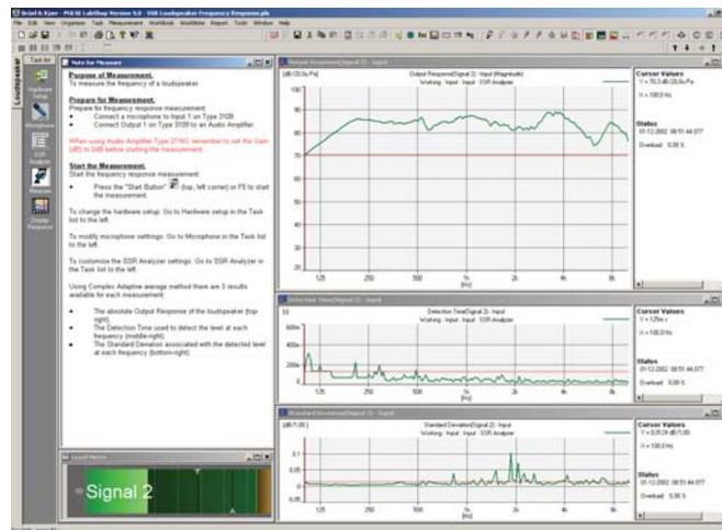
A number of specific parameters can be used to characterize an electroacoustic device. The most commonly used parameters to characterize the static performance of an electroacoustic device are: output response, frequency response, harmonic distortion, intermodulation distortion, difference frequency distortion and directivity. In a similar way, the dynamic behaviour of an electroacoustic device can be described by attack and decay time, switching time and attenuation, etc.
