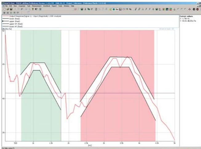
PULSE audio analyzers also support post-processing of measurement results. Data can be post-processed in real-time using PULSE language or Microsoft Excel, and a dynamic link to the measurement data adds to the flexibility of post-processing. Special types of post-processing such as tolerance checking can be performed live on the measurement, resulting in the display of a clear pass-fail verdict, and an event that can be used to trigger a specific handling.
