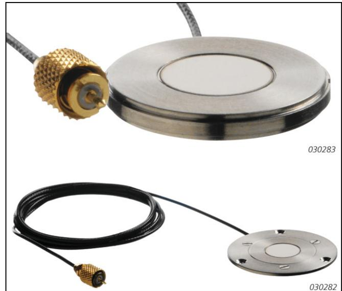
The microphone offers high mounting flexibility and its diaphragm is flush with the microphone housing in order to minimise the microphone's wind-generated noise. The microphone's pressure-equalisation vent is placed just next to the diaphragm on the front of the microphone; this is important as static pressure can vary rapidly with position in the applications for which the microphone is designed.
